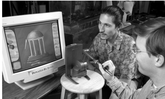
Figure 26.1. Haptic painting system setup: an artist using a haptic stylus to paint directly on the virtual canvas using dAb. (© 2002 IEEE)
