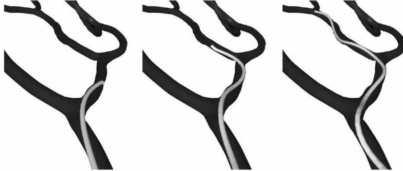
Figure 20.8. Catheter navigation inside the cerebrovascular network. Complex, nonlinear deformations are correctly represented by an incremental FEM model. Collision detection and collision response allow the catheter to stay within the lumen of the vessels.
