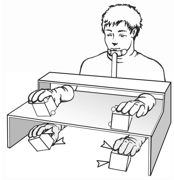
Figure 2.5. Schematic view of the experimental set-up in Pavani et al.'s [Pavani et al. 00] rubber hand experiment, highlighting the location of the vibrotactile stimulators (indicated by the four arrows) on the foam cubes held by the participant below an occluding screen, and the visual distractor lights (four open circles on the upper cubes) held by the rubber hands that, when present, were aligned with the participant's own hands. Note that in some conditions (not shown), the rubber arms were placed at 90 degrees with respect to the participant's own arms (i.e., in a posture that the participant could not possibly adopt).
