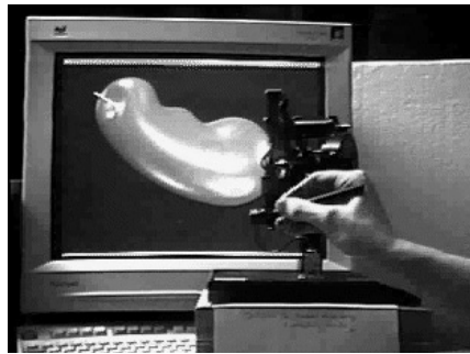
Figure 19.10. Photograph of simulation in use. Users were able to push, slide, and pull on the surface of the model using a point-like manipulandum.
