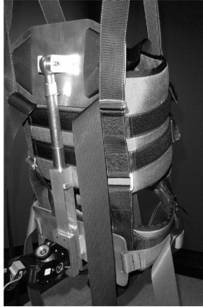
Figure 5.5. Body weight support harness integrated with the mechanism-based harness.
