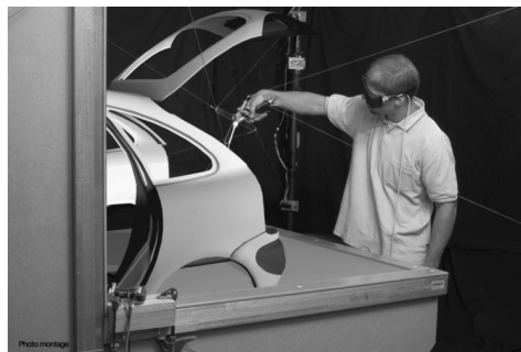
Figure 22.9. Putty application © PSA Peugeot Citroën.
