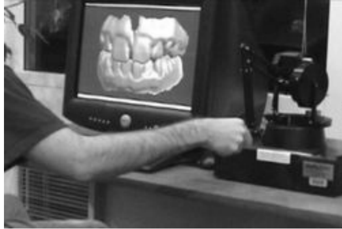
Figure 8.1. Manipulation of a virtual jaw. The user manipulates a haptic device, and though the rendering algorithm can perceive forces as if manipulating the upper jaw in the virtual environment.
