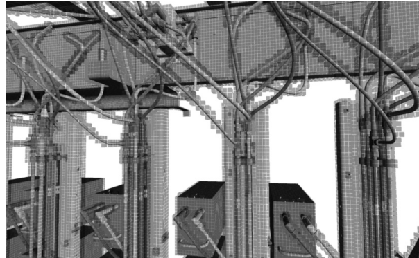
Figure 11.7. Close-up features of a wiring and hydraulic installation in which many objects are merged into a single voxmap (shown as semi-transparent cubes). The voxel size is artificially inflated for illustration purposes.
